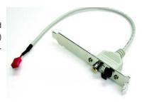
Connect the SPDIF output device to the rear bracket of PC, and fix it with screw.
