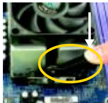
Figure 4 & 5. Alignment of heatsink assembly with standoffs.
