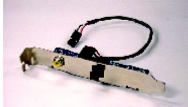
1. Connect the SPDIF output device to the rear bracket of PC, and fix it with screw.
